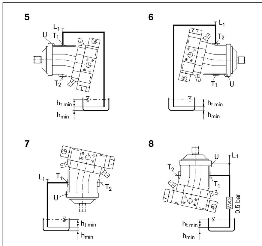
Fig. 7: A6VM above-reservoir installation - with installation position 5–8
